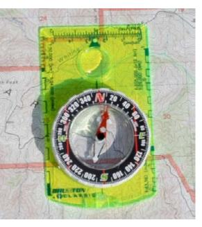
Now if we needed to travel between Montara Knob and North Peak the simple thing to do is follow the bearing indicated by the compass. In this case that may not be the most efficient route but the same procedure would apply to any 2 map points, features or waypoints you choose.
